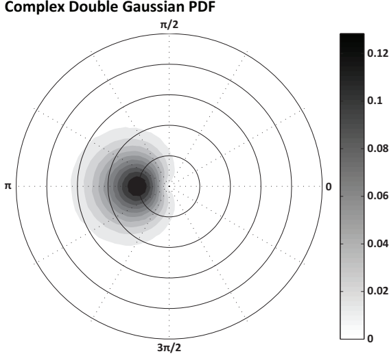
Fig. 1. Plot of the two-dimensional PDF f_{R_z, \Theta_z}(r_z, \theta_z) , described in (1), for k_x = 1, k_y = 1/\sqrt{2} and \phi_x = \phi_y = \pi/2 .
